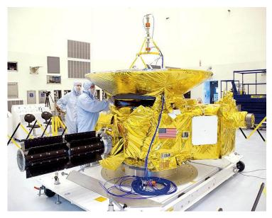
New Horizon Space Probe, in assembly before launch. The black tube is the thermoelectric-radioisotope generator. NASA
