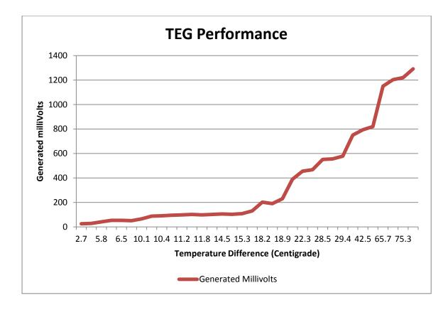
As can be seen, the results look non-linear because there are more measurements done with a small temperature difference than a large temperature difference. The adopted solution to this problem was to pick a temperature interval of 5 degrees Centigrade and scale and then average all the measurements within each 5-degree range, i.e. 0-5, 5-10, 10-15, etc.
