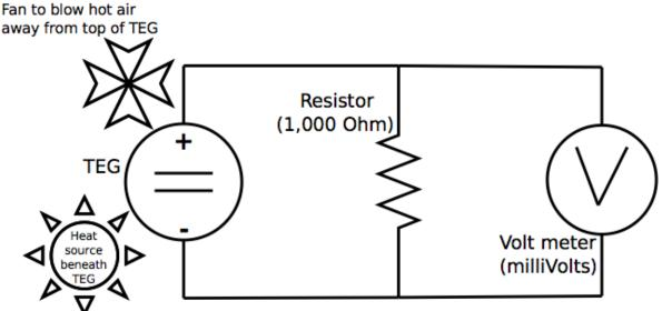
Measure volts and calculate power (Watts)
