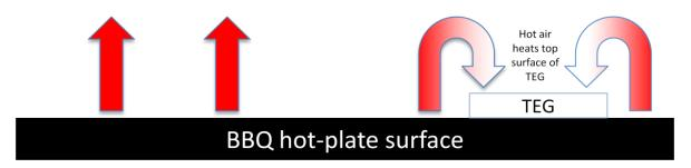
To counter this possibility, all the following TEG experiments incorporated a fan blowing over the top of the experiment to try to stop convection currents. This seemed to help, because later measurements showed more of a temperature difference between the top of the TEG and the BBQ or frypan surface.
